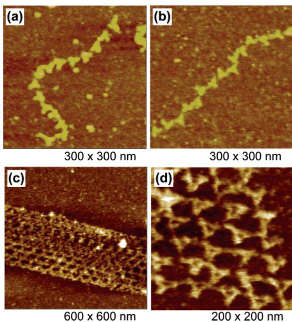
**Figure 3.** AFM images of DNA triangle arrays: 1D arrays with a periodicity of 7 (a) and 7.5 turns (b), and 2D arrays (c and d).
